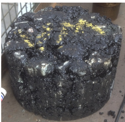
Figure 5: Example for disintegration and unfilled voids on Marshall specimen WA1 (AC 45 T S)
