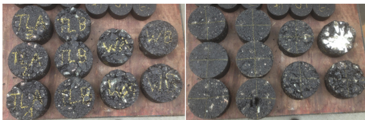
Figure 2: Upper (left picture) and under side (right picture) of selected Marshall specimens (left in each picture AC 45 B/T S, right AC 45 T S, WB1 shows residues of filter paper)
