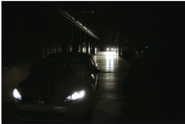
Fig. 32: Test set-up: The following vehicle at a distance of 50 m with turned on dipped beam head lights
