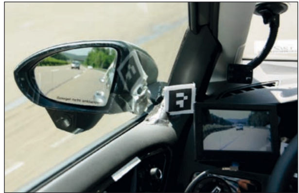
Fig. 18: Difficult to detect vehicle in the background (white vehicle on beige concrete carriageway)
