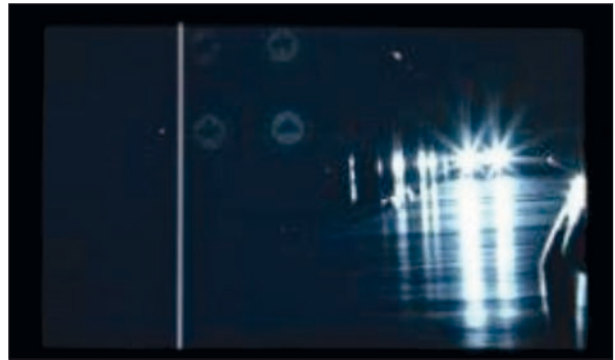
Fig. 35: Monitor at a distance of 50 m and turned on high beam head lights
