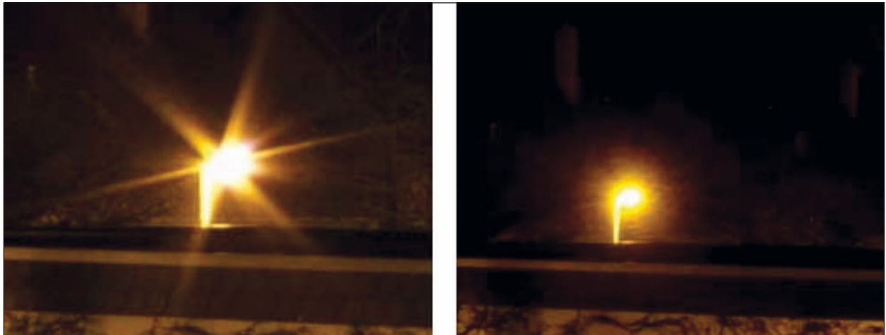
Fig. 11: Flare effect (left small aperture, right large aperture)
