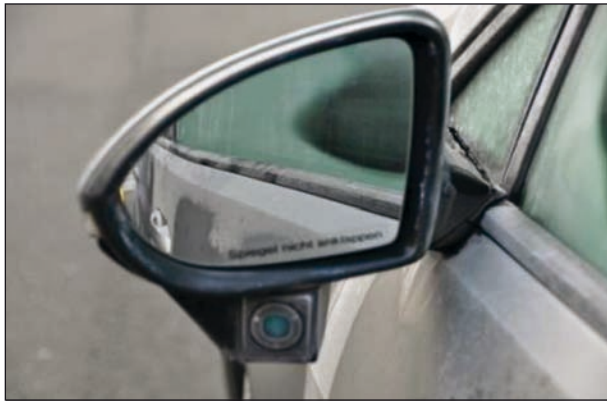
Fig. 45: Mirror is clear, camera still shows condensation
