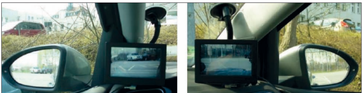
Fig. 6: Integration of the monitors next to the A-pillar (Position CMS 3)
