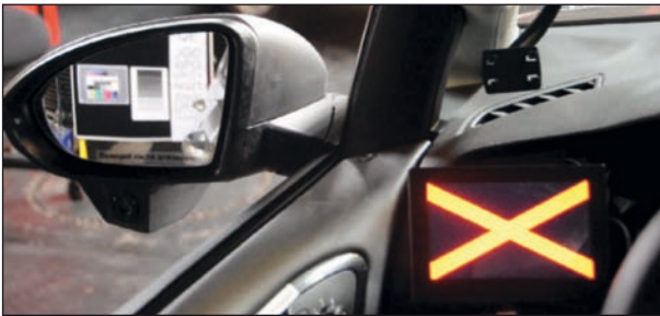
Fig. 41: Loss of image caused by electromagnetic radiation
