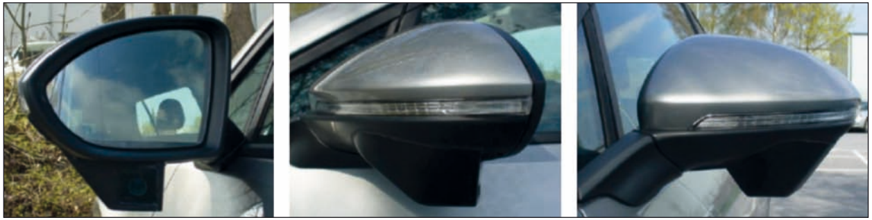
Fig. 3: Left exterior mirror with camera mounted to the mirror housing
