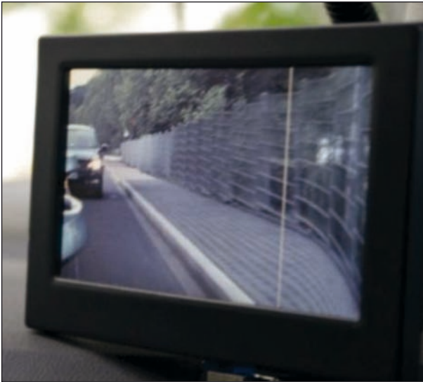
Fig. 8: Right-hand monitor with aspherical section
