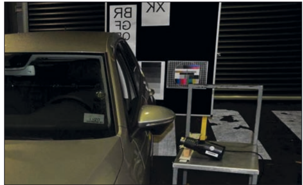
Fig. 47: Test set-up for behaviour in extreme heat
