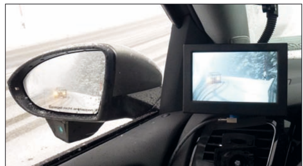
Fig. 27: Comparison at snow fall and higher ambient luminance (distant vehicle)
