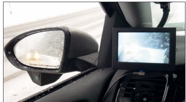
Fig. 26: Comparison at snow fall and higher ambient luminance (close vehicle)
