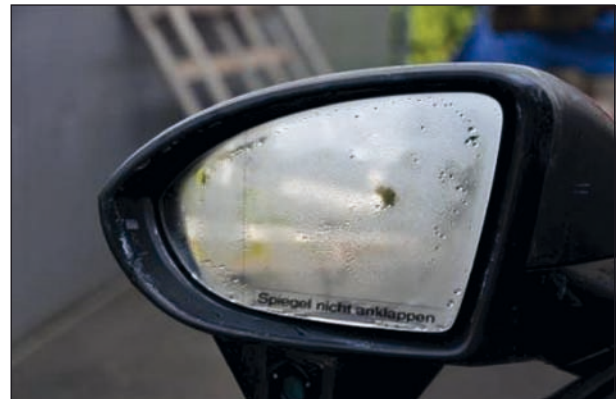
Fig. 44: Camera and mirror fogged up
