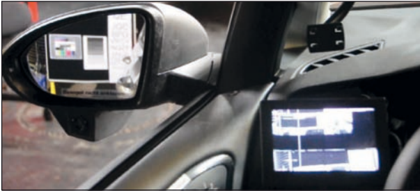
Fig. 40: Error in image caused by electromagnetic radiation
