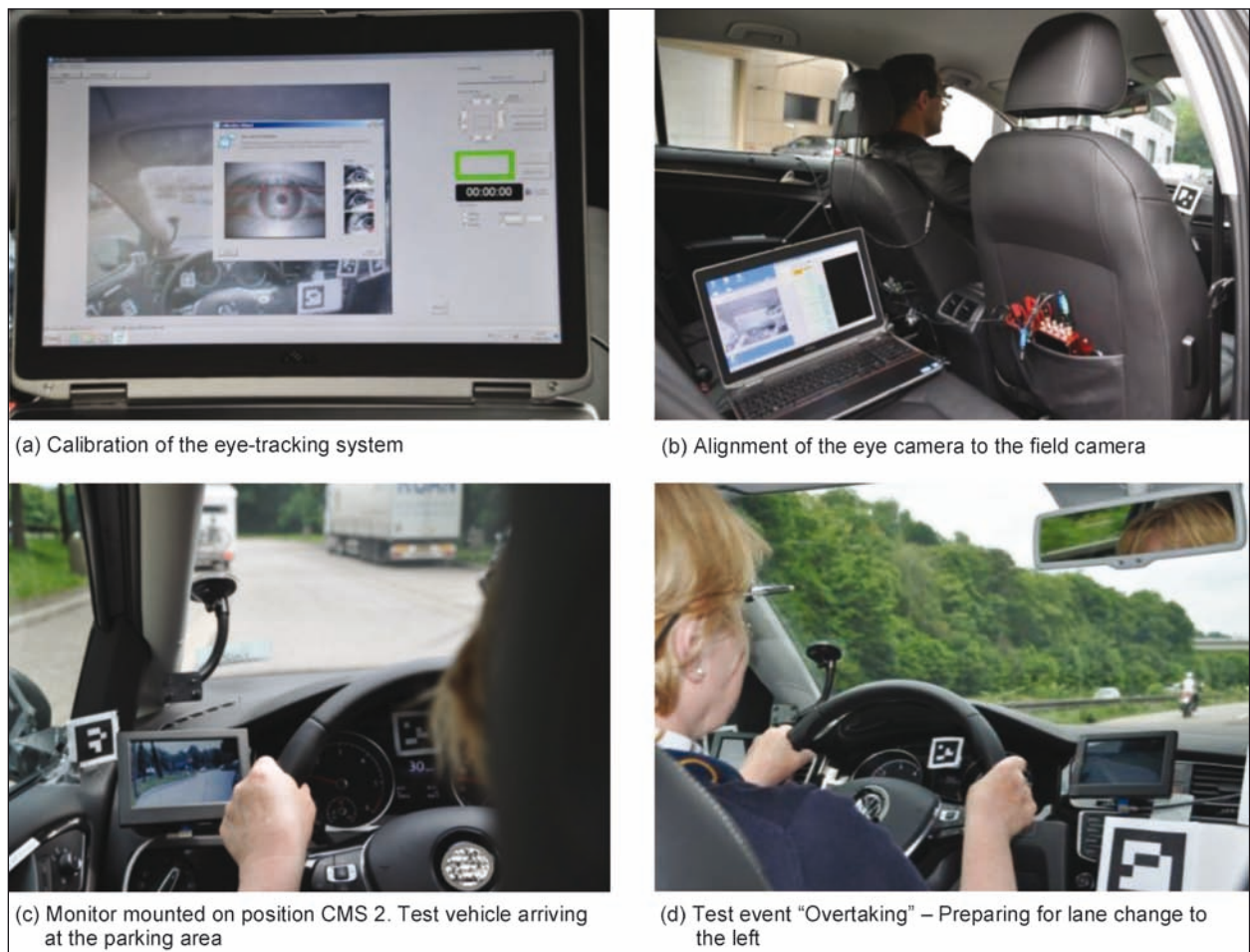
Fig. 60: Measuring glance behaviour by using an eye-tracking system
